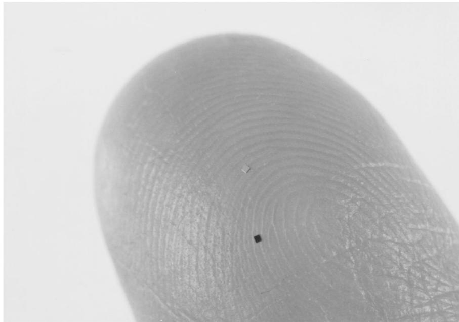
**Note:** The  $\mu$ -chip uses the frequency of 2.45GHz. It has a 128-bit ROM for storing the ID with no write-read and no anti-collision capabilities. Its unique ID numbers can be used to individually identify trillions of trillions of objects with no duplication. Moreover with a size of 0.4mm square, the  $\mu$ -chip is small enough to be attached to a variety of minute objects including embedding in paper
