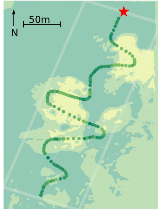
Figure 3: Resulting map of surface material. Gaussian process inference extrapolates from sparse samples by leveraging remote sensing and proximity correlations. The rover dynamically adapts its path to visit areas for which predictions are uncertain, and ignores the homogeneous area to the upper left.
