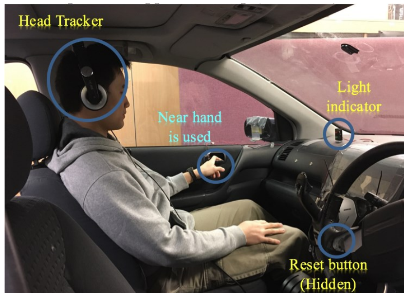
Figure 3. Participant seated in the passenger side of the 2001 Honda Civic, showing head-tracker, LED indicator and location of reset button.
