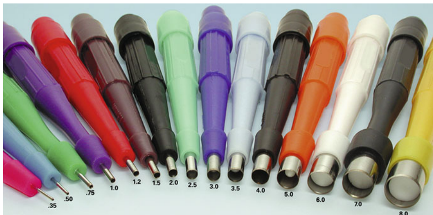
Fig. 4.2 Harris Uni-Core punching tools of different diameters for manual punch (with permission from Ted Pella, Inc.)
