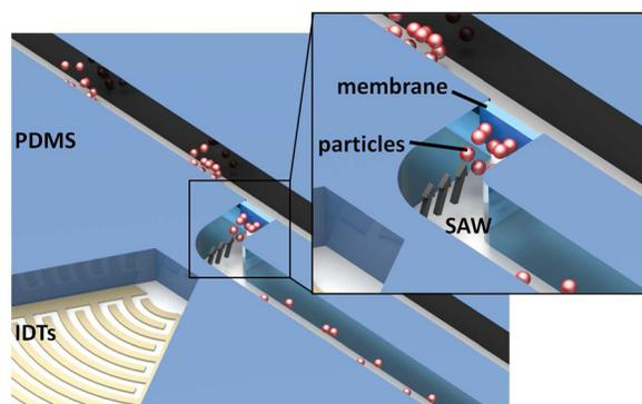
FIG. 1. Controlled release concept: a SAW generated by a series of focussed IDTs on a piezoelectric substrate generates an acoustic field that imparts a force, mostly in the vertical direction, against particles in a fluid flow. Without SAW applied, particles pass through the gap under the membrane unimpeded. However, subject to this force, particles are unable to pass beyond a microfabricated PDMS membrane in their path. This methodology enables on-demand particle concentration and release.
