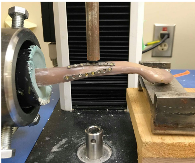
Fig. 2 Anterior–posterior view of three-point bending testing. Load cell located immediately lateral to fracture site
