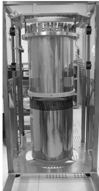
Fig. 7. Two electrodes fixed on the vertical insertion system used to assembly the detector.
