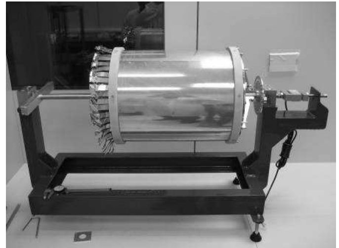
Fig. 8. The chamber mounted on the support system and stretched. The tension is measured by the load cell on the right end.
