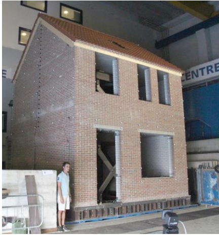
Figure 3. EUC-BUILD1: shake-table test specimen and corresponding damage pattern at end of testing on both outer-leaf clay walls and inner-leaf calcium-silicate walls (Graziotti et al. 2015, 2017)
