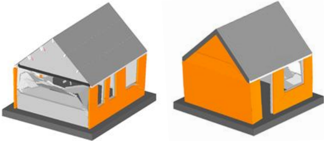
Figure 9. LNEC-BUILD1: specimen collapse mode as reproduced by AEM model
