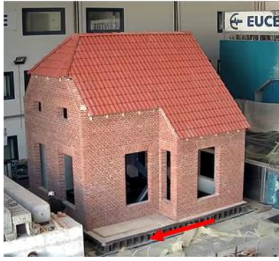
Figure 10. EUC-BUILD2: shake-table test specimen and corresponding damage pattern at end of testing (Graziotti et al., 2016)
