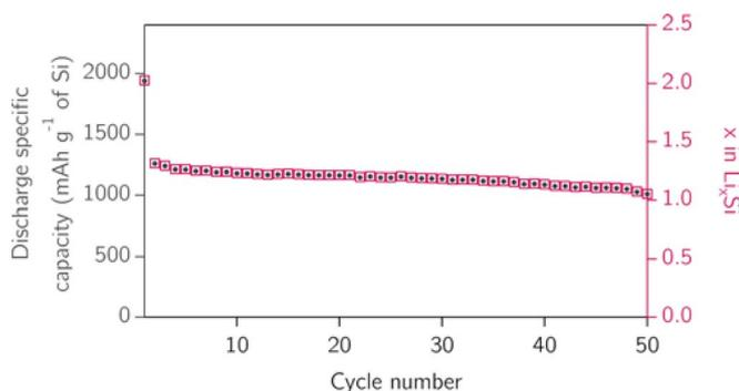
**Figure 4.** Moles of Li per Si or specific capacity of Si in the Sn:Si:SSE anode in Figure 1. The value is developed assuming Sn fully lithiates every cycle.
