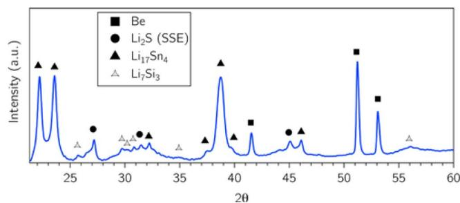
**Figure 3.** (a) Ex-situ XRD spectrum of Sn:Si:SSE anode discharged to 5 mV vs. Li. Sn fully lithiates to  $\text{Li}_{17}\text{Sn}_4$  phase. In-situ derived pressure from Sn expansion allows Si to crystallize to the  $\text{Li}_7\text{Si}_3$  phase rather than remaining in the amorphous analogue.
