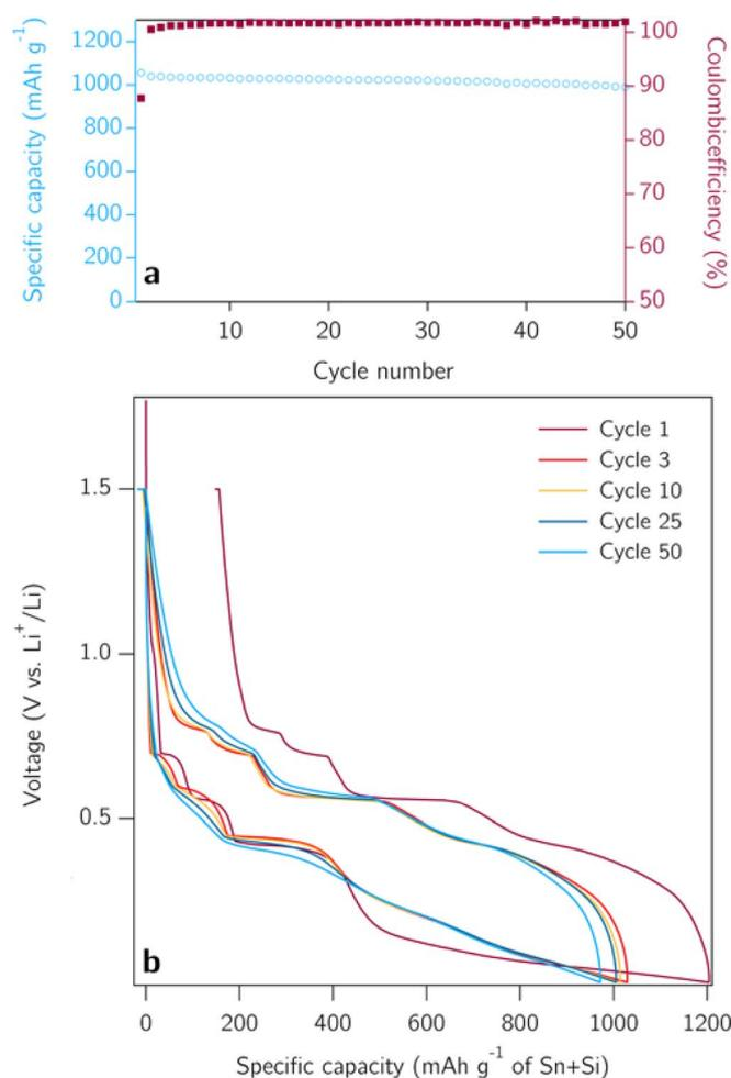
**Figure 1.** (a) Cycle performance and coulombic efficiency of Sn:Si:SSE [7(3:1):3] anode in an all-solid-state Li-ion battery at 60°C with a C/20-rate (80 mA g<sup>-1</sup>) and (b) Corresponding voltage profiles of the Sn:Si:SSE anode vs. LiIn counter electrode (converted to vs. Li).
