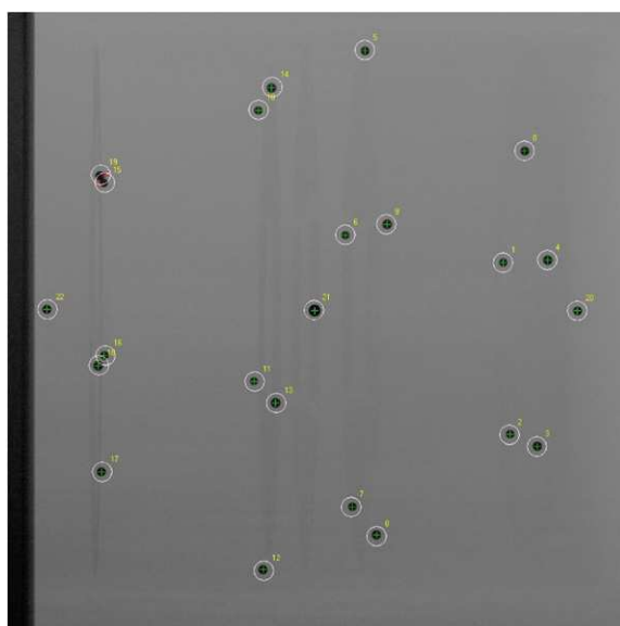
Figure 4. A calibration image, showing the metal balls in the dodecahedron phantom. The crosses on top of the balls identify the successfully recognized balls. As can be seen from the image, ball numbers 15 and 19 were failed to identify properly (due to overlap). The white circles represent the back-projected dodecahedron corners after the dodecahedron was fitted to the image. The dodecahedron position in 3D space can even be determined when a few balls are missed.
