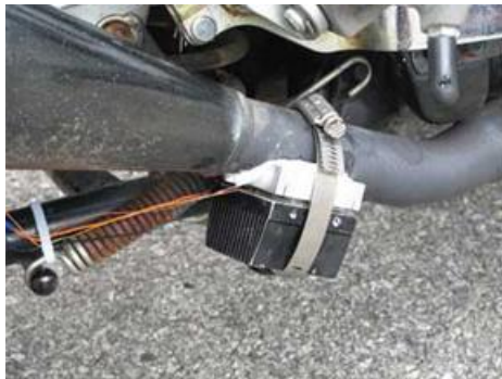
Figure 4. The TEG mounted on the exhaust pipe of the Ninja 250R
