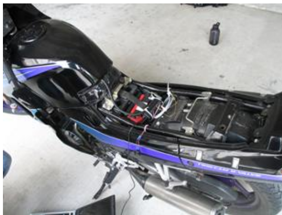
Figure 5. The Pace Scientific, Inc. XR5-SE-M-50mV data logger mounted underneath the seat
