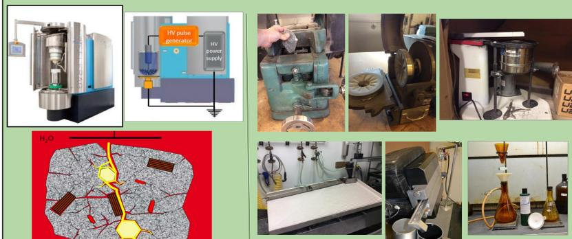
Images (selective fragmentation): Top left - Image of the Selfrag Lab used to reduce samples. Top right - cross-sectional view of the Selfrag Lab showing high-voltage pulse being introduced to the processing vessel. Bottom - Illustration showing the discharge track as it travels through the material following natural boundaries.
