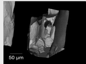
Selective fragmentation fraction (Temora 2): BSE image of fractured zircon grain fractured at the contact of two inclusions. See illustration (right).
