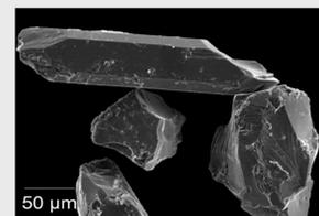
Traditional fraction (Temora 2): SEI image of fractured zircon grains with plagioclase intergrowths at the surfaces.
