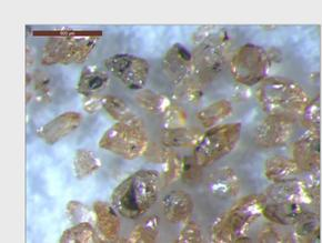
Traditional fraction (Temora 2): Reflected light image of liberated zircon grains. Note that nearly all inclusions have remained within the zircon grains.
