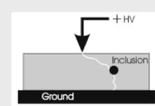
Illustration of the preferential attraction of the discharge track to metallic, or high dielectric constant, inclusions (as evidenced by the image to the left.)
