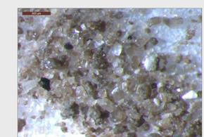
Selective fragmentation fraction (CO-ML-L1): Reflected light image of carbonate rock material. Note the fragments of microfossil (dark grains) and euhedral calcite grains.
