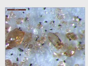
Selective fragmentation fraction (Temora 2): Reflected light image of zircon grains liberated. Note the near absence of in-place inclusions, of which can be seen lying around the zircon grains.
