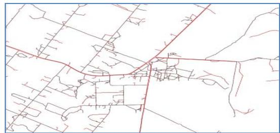
**Figure 15:** result of v.generalize algorithm, using network method of generalization operation in Qgis for representing roads for scale of 1:10,000
