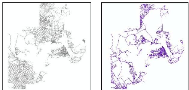
**Figure 16(a, b):** Before and after applying Collapse Dual Line to centerline tool (zoom 1:250,000)
