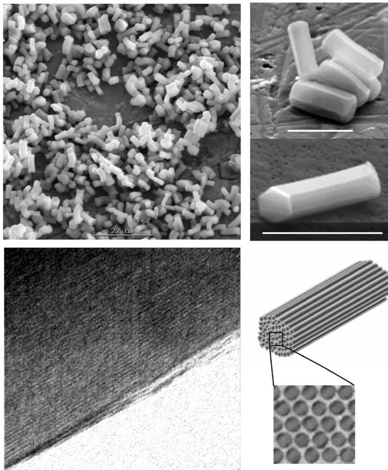
FIG. 1. Top: Scanning electron microscopy image of parallel nanochannels in fiber like ASNC of uniform shape. A large area (left bar size is  $22 \mu\text{m}$ ) and zoom to a few ASNC (right, bar size is  $5 \mu\text{m}$ ). Bottom: TEM image of near the ASNC edge showing a periodicity of about  $3.6 \text{ nm}$  (left); a schematics showing the arrangement of nanochannels in silica matrix (right).
