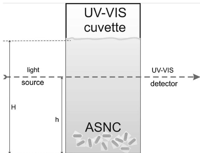
FIG. 2. Schematics of the measurements of the concentration of the dye diffusing out of the nanochannels of ASNCs. Dye concentration in the cuvette was measured by using Beer's law, which relates the concentration and absorbance.
