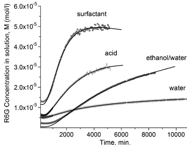
FIG. 3. Measured concentrations of the dye molecules diffused out of ASNCs in water, 1 mM surfactant solution, 25% ethanol in water solution, and acidic aqueous solution with pH 1. Solid lines are the model [Eq. (3)] fits. The initial number of molecules per nanochannel is found by multiplying  $\Lambda_0$  by the volume of each ASNC.
