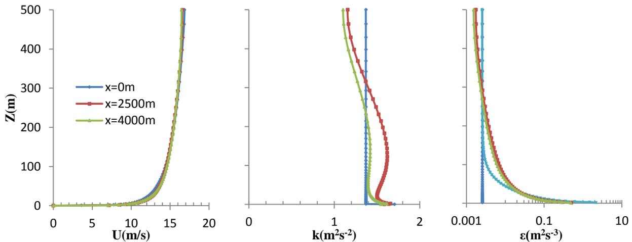
Figure 5. Plots of velocity, turbulent kinetic energy and turbulent dissipation for case 2.4
