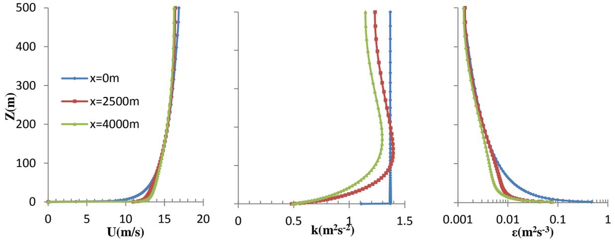
**Figure 2. Plots of velocity, turbulent kinetic energy and turbulent dissipation for case 2.1**
