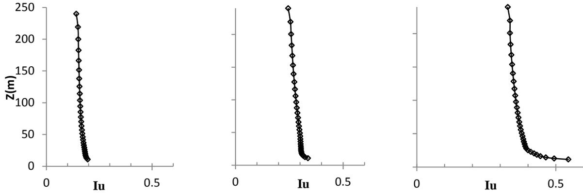
**Figure 7. Normalized wind speed and turbulence intensity profiles for open-country (left), suburban (middle), and urban (right) roughness.**
