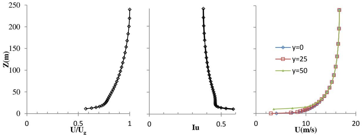
**Figure 8. Average normalized wind speed, average turbulence intensity profile and wind speed at three sections of a three patch Urban-Suburban-Urban roughness.**
