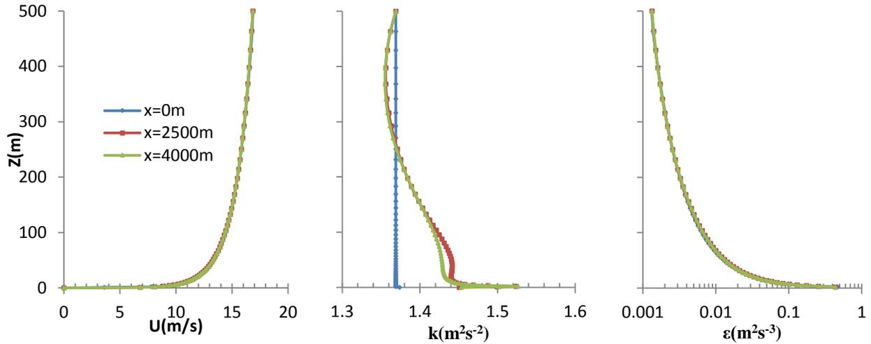
Figure 4. Plots of velocity, turbulent kinetic energy and turbulent dissipation for case 2.3
