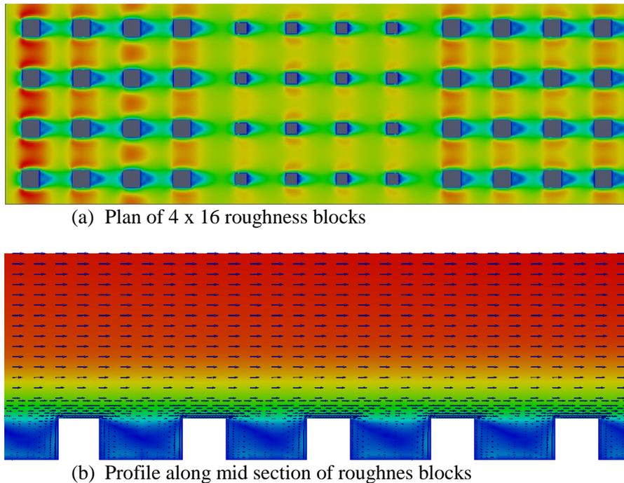
**Figure 6. Mean velocity profile for a three patch roughness elements (k-epsilon model).**
