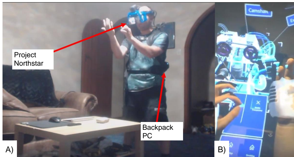
Figure 1: We present Project Esky, an eXtended Reality (XR) framework that enables high fidelity XR content on any hardware configuration. A) A user wearing an OST-HMD with a 6DOF head tracker, hand tracker, and PC is able to develop high fidelity experiences with hand-gesture interactions. B) An image through the lens of the OST-HMD, showing a user interacting with the engine e-learning example displayed in the accompanying video.
