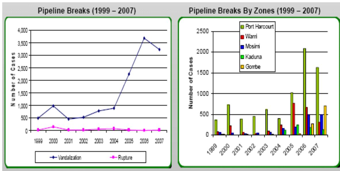
**Figure 1a/b: Vandalism/interdiction trend against rupture/corrosion (1999-2007)**
