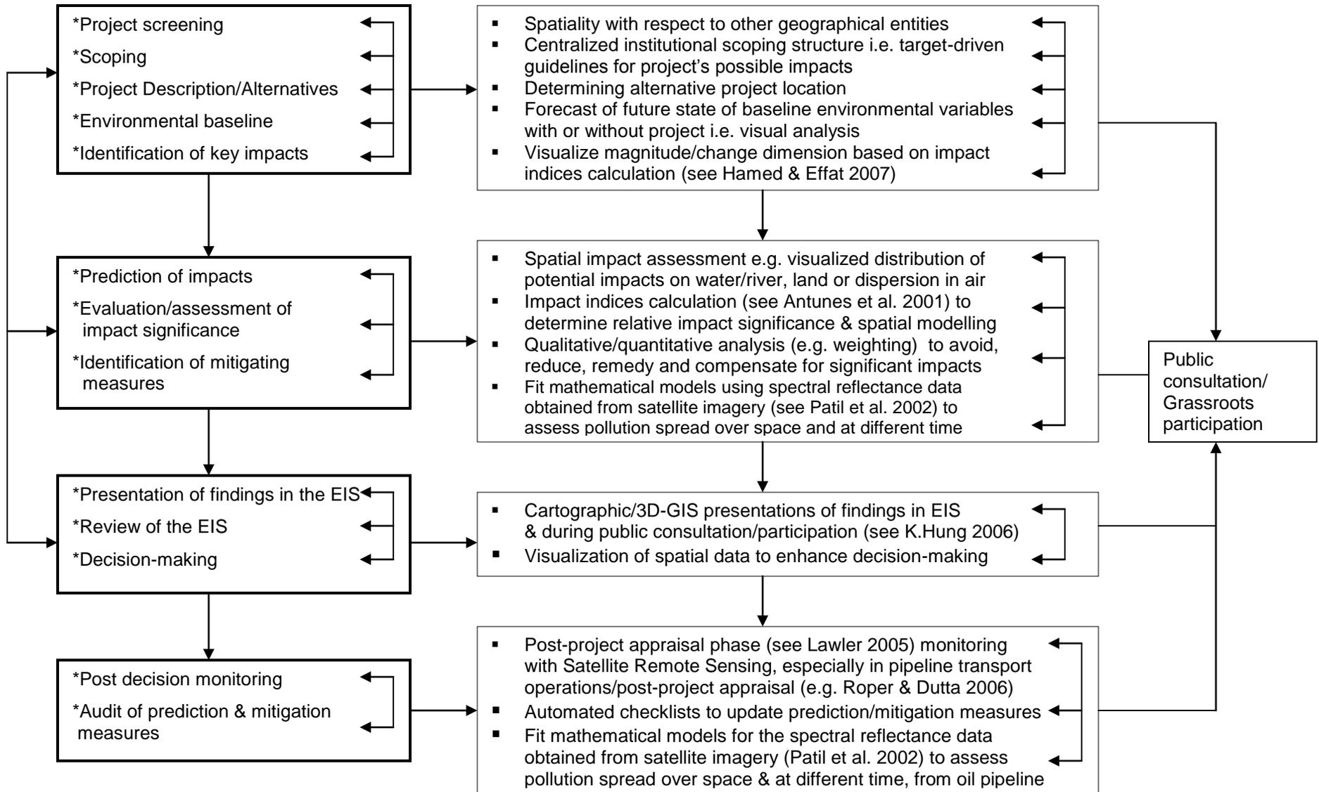
**Figure 6: Schematic view of proposed EIA methodology & procedure**
