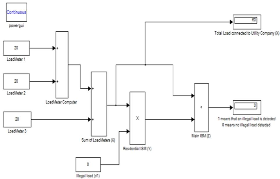
Figure 9: Simulink simulation of the anti-theft metering system.
