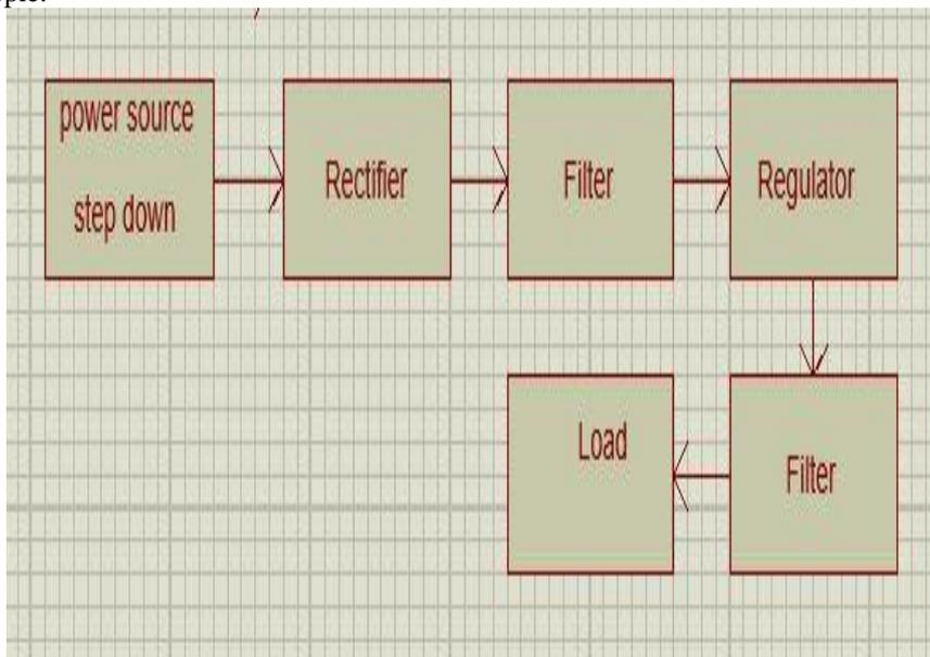
Figure 4: Block diagram of the power supply unit
