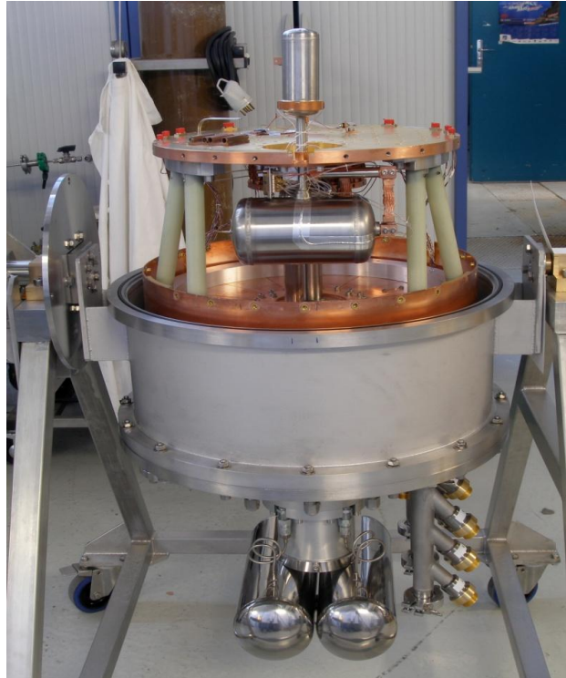
Figure 6: Cryo-cooler inside the Cryolic cryostat.
