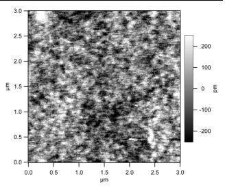
Fig. S3 Atomic force microscopy surface scan of the SBN60 thin film surface over a 3  $\mu$ m × 3  $\mu$ m area.
