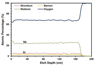
Fig. S1 X-ray photoelectron spectroscopy depth profile of  $\sim$ 175 nm thick SBN60 film, as-deposited under conditions in Table S1.
