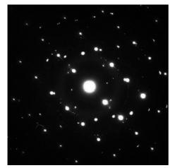
**Fig. S2** Selected area electron diffraction pattern from the SBN60-STO film-substrate interface. The indexed versions of this as-collected pattern are presented in Fig. 3.
