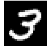
Figure 5. Example of a MNIST input. An image is passed to the network as a matrix of 28 by 28 floating point numbers, with a value varying from 0 to 1.
