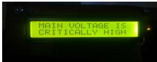
Figure 14. Screen display upon occurrence of overvoltage
