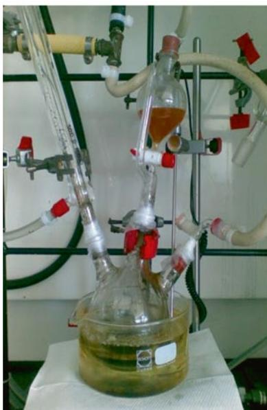
**Fig. 2** A reflux system for synthesis of superparamagnetic iron oxide nanoparticles (SPIONs). (A) Heating magnetic stirrer, (B) temperature controller, (C) water-cooled condenser, (D) water-cooled condenser, (E) air evacuation vacuum pump
