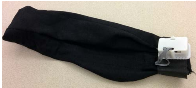
Figure 2: Plastic hoops incorporated in this prototype were incorporated to hold the NIR sensors away from the nylon netting.
