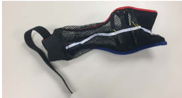
Figure 2: Plastic hoops incorporated in this prototype were incorporated to hold the NIR sensors away from the nylon netting.
