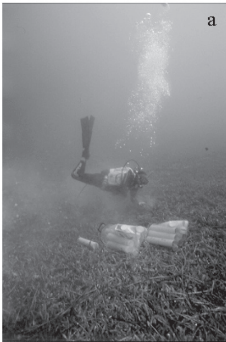
Fig. 6 - Sampling by corer samplers used by SCUBA divers: a) on soft bottoms near a Posidonia oceanica meadow (Photograph by A. Floris). b) in a brackish environment (Photograph by S.E.L.C.).
