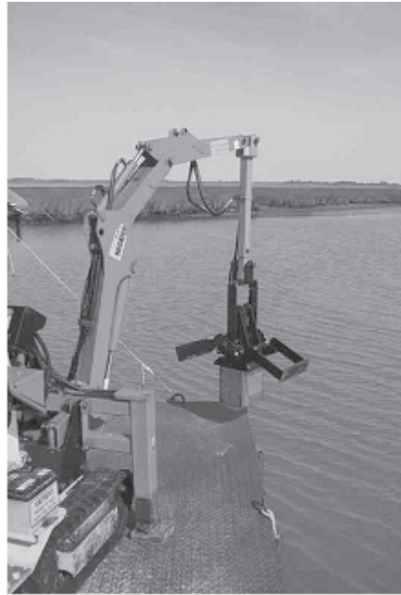
Fig. 2 - Ekman grab, modified by Pessa, used in Venice Lagoon (Photograph by G. Pessa).
