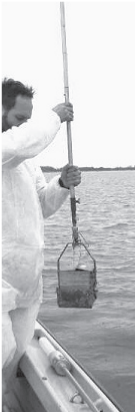
Fig. 3 - Modified version of Ekman-Birge grab suitable for manual sampling in the littoral zone or at shallow depths (1-1.5 m).
