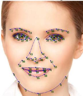
Figure 11: Facial Features detected by Luxand Face SDK.
