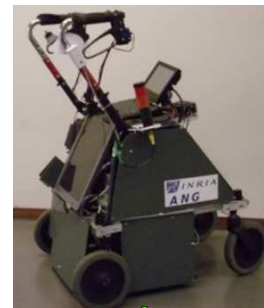
Fig. 6. The Assisted Navigation Guide (ANG walker) [34] is equipped with various sensors and a bistable clutching mechanism
