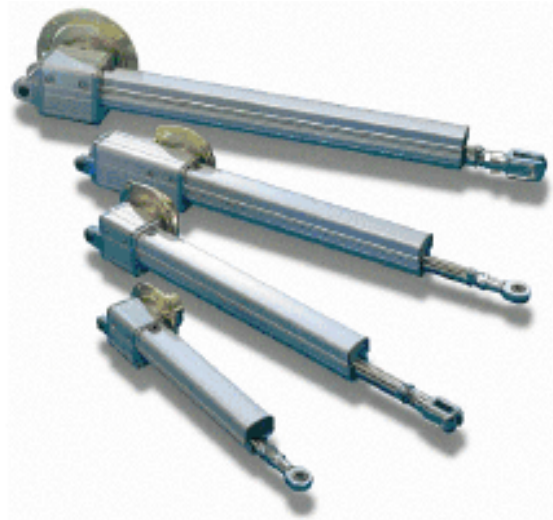
Figure 2. An assortment of linear actuators. Linear actuators work by turning a threaded rod with an electric motor. The threaded rod in turn extends the actuator arm from the actuator's case. In the figure, the arm is the narrow end of the actuator.
