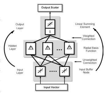
Fig. 2. Schematic of the radial basis function (RBF) neural network
