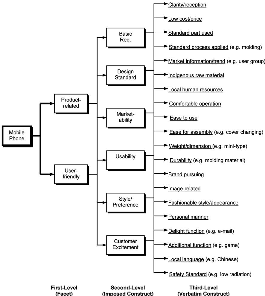
Fig. 3. Graphic representation of ladder-ing for mobile hand phone design
