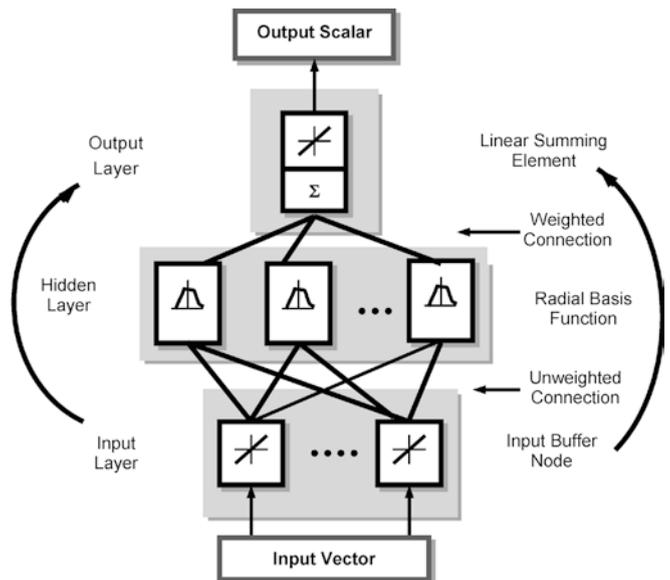
Fig. 2. Schematic of the radial basis function (RBF) neural network
