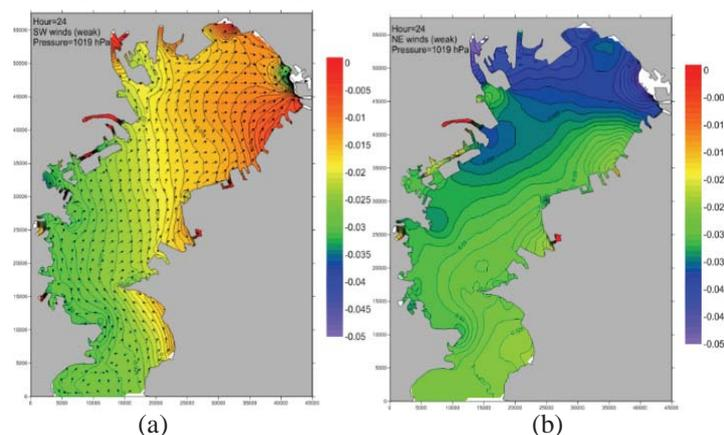
3. **Figure 3** Model H: Spatial distribution of the free surface elevation due to storm surge in Tokyo Bay,
