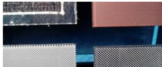
Figure 3: Close-up photo of the various CIGS panels of the prototype demonstrator. At the top left the black textured glass panel is depicted, at the top right the printed red panel, at the bottom left the printed grey panel and at the bottom right the grey foil panel.
