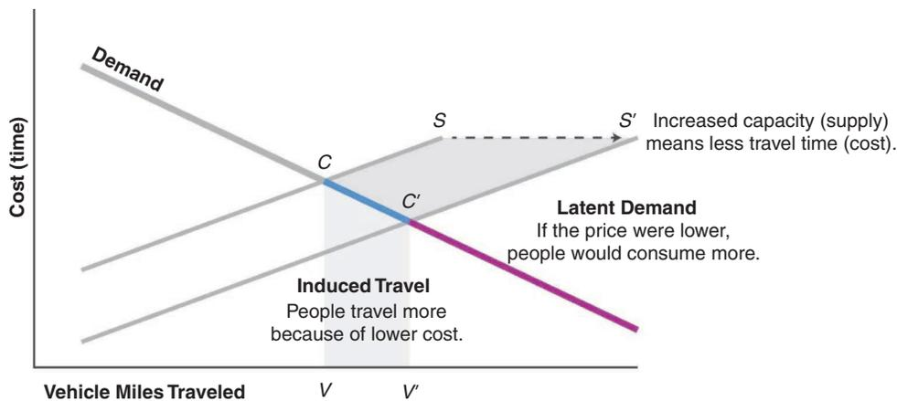
FIGURE 2 Supply and demand relationships for induced travel ( $C$  = initial cost;  $C'$  = new cost;  $S$  = initial supply/capacity;  $S'$  = new supply/capacity;  $V$  = initial VMT;  $V'$  = new VMT).
