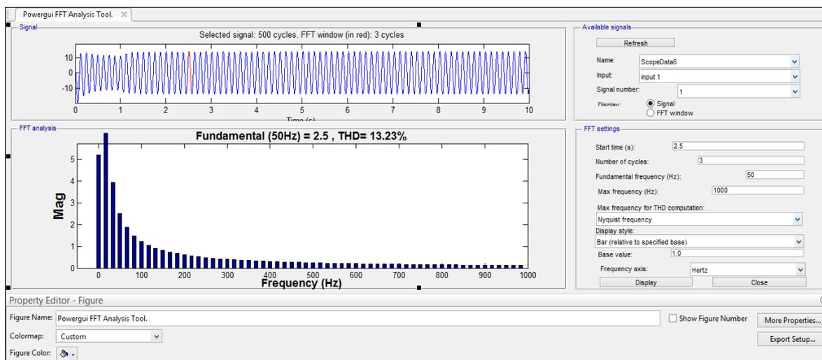
Figure 6: The Current Spectral examination of the harmonic distortion.
