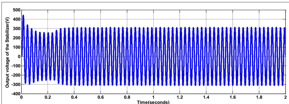
Figure 4: Waveform of the Output voltage of the proposed system.
