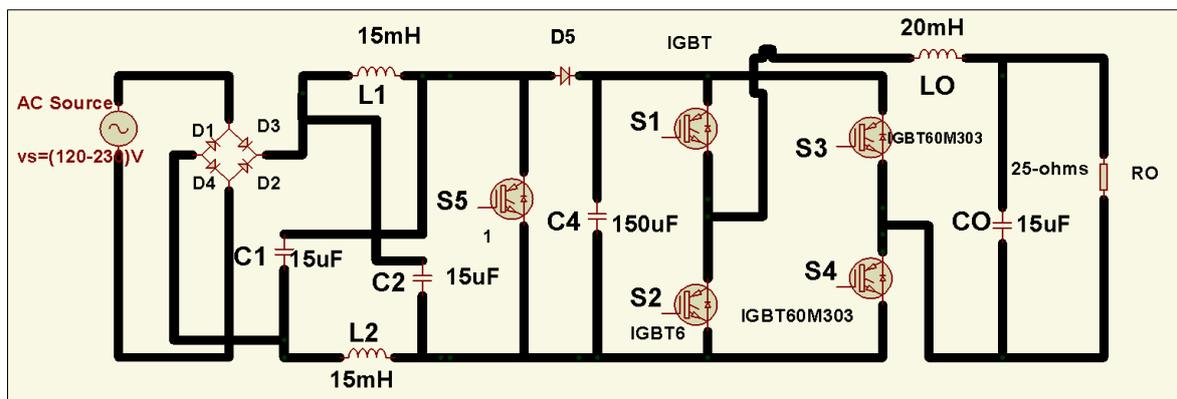
Figure 1: Circuit topology of the proposed improved system.
