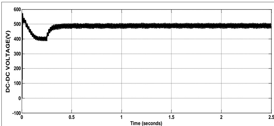
Figure 3: Waveforms of the input voltage and the boosted voltage of DC-DC converter.
