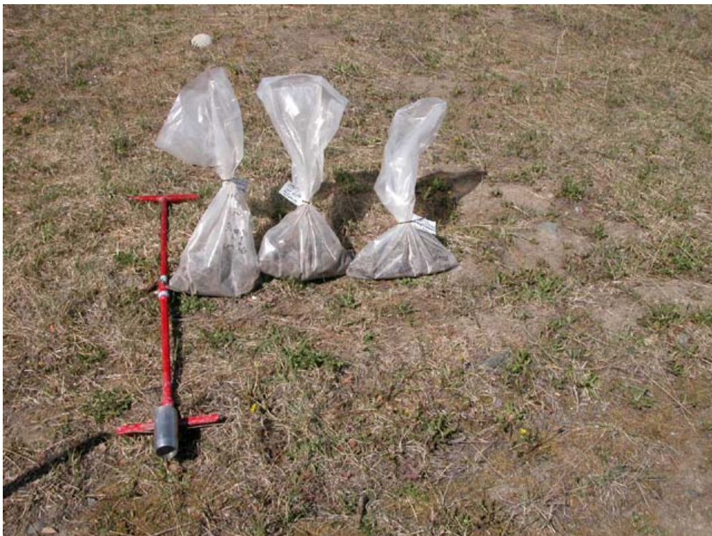
c. Triplicate multi-increment samples. The mean NG concentration was 132 \mu\text{g/g} .
