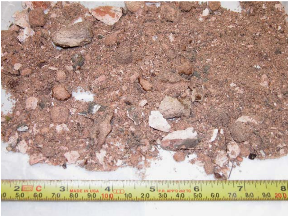
d. HE residue from low-order detonation. The 18 HE chunks were friable and were reduced to much smaller particles when collected for weighing.
