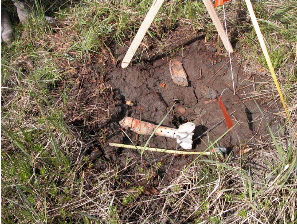
a. Crater, tail assembly, scrap, and HE chunks at impact point.
