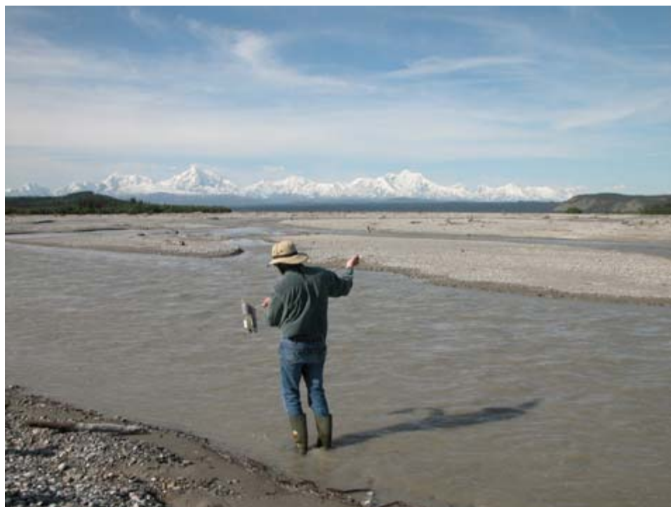
c. Water sampling downstream of berm using a US DH-48 depth-integrating suspended sediment sampler.
