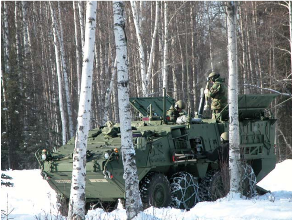
a. Member of the 4 th /23 rd Infantry Regiment preparing to fire a projectile from a 120-mm mortar (M121) mounted on an M1129 Light Armored Vehicle III Stryker at FP Fox.
