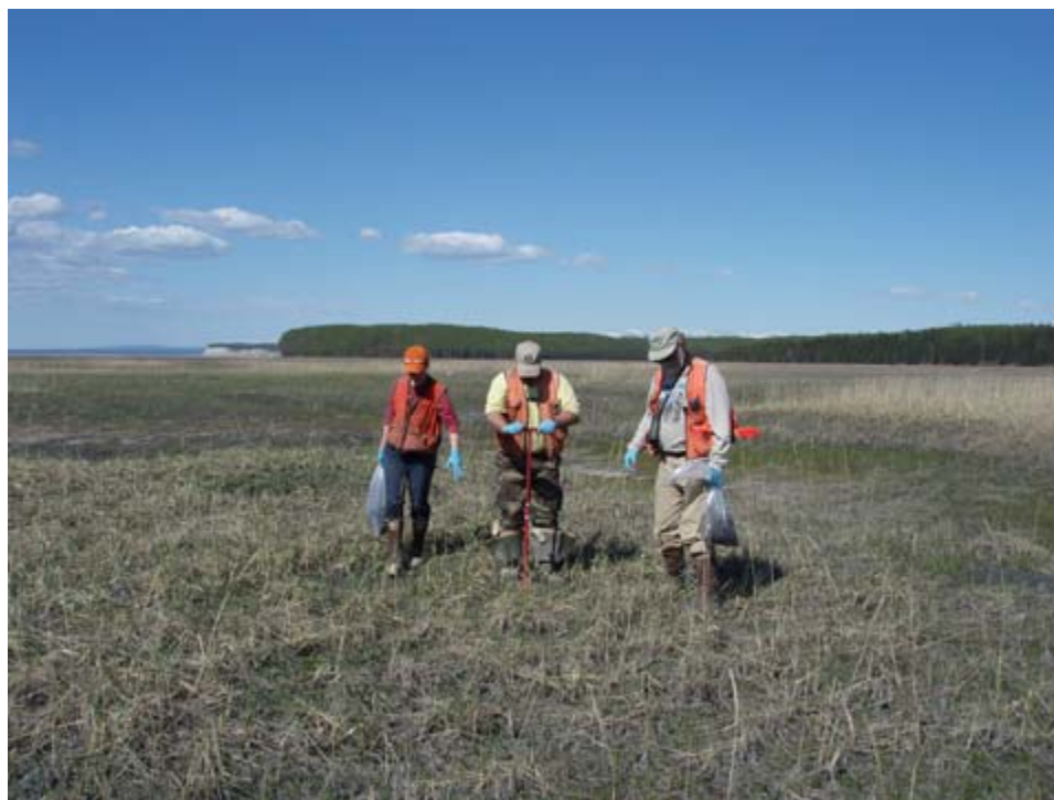
Figure 17. Field sample collection within a 30-m \times 30-m area encompassing a 120-mm mortar projectile low-order detonation. Multi-increment samples were composed of approximately 100 cores (4.75-cm ID) collected to a depth of 3 cm.
