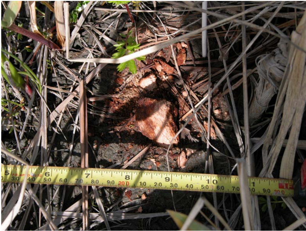
c. Close-up of one of the HE chunks from the low-order detonation.
