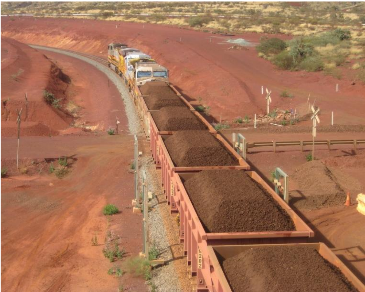
Typical fully laden iron-ore rail truck
