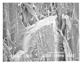
Figure C. SEM of Failure Surface from ASTM D-2559 Specimen
