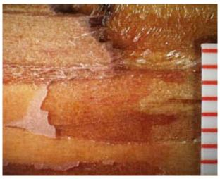
Figure B. Failure Surface with Stain from ASTM D 2559 Specimen
