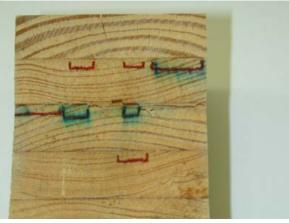
Figure A. Failure in ASTM D 2559 Specimen Bonded with Epoxy
