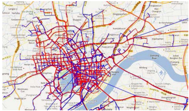
Fig. 2. Traces of a taxi in Hangzhou city during a month, where red or blue indicates the taxi is occupied or vacant.
