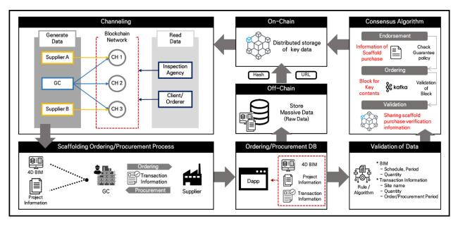
Figure 2. Blockchain-based scaffolding management process and key features
