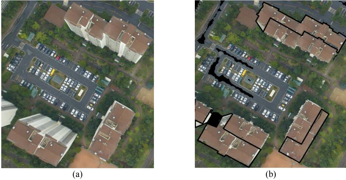
Figure 1. Perspective image (a) and corresponding ortho-photo (b) with double mapped areas enclosed by solid black lines
