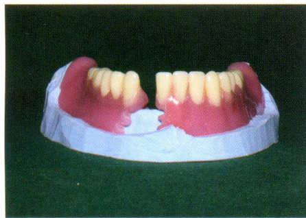
Figure 16 Denture segments positioned on putty cast. Space created for the repair resin
