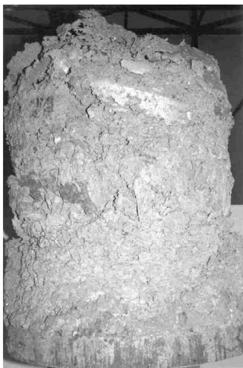
Fig. 4 : Titanium sponge cake weighing about 3000 kg
