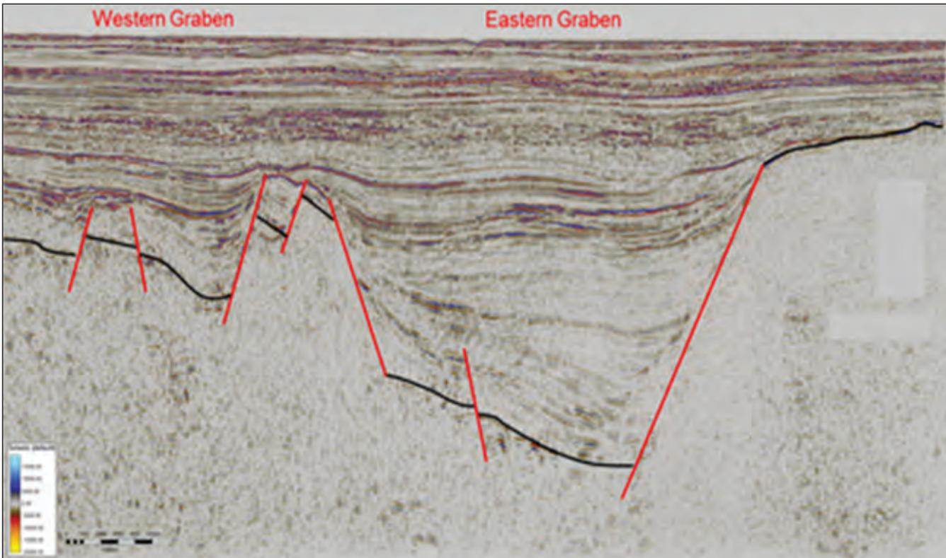
**Figure 1.** North Falkland Basin Failed Rift System
