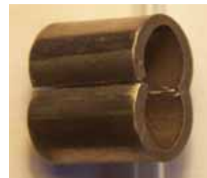
图 4 650°C、30%压缩比条件下试样的破坏图片 Fig.4 Collapse of a specimen under loading with 30% compression ratio at 650
