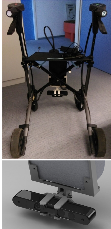
Fig. 1. A rollator with propose add-on camera
