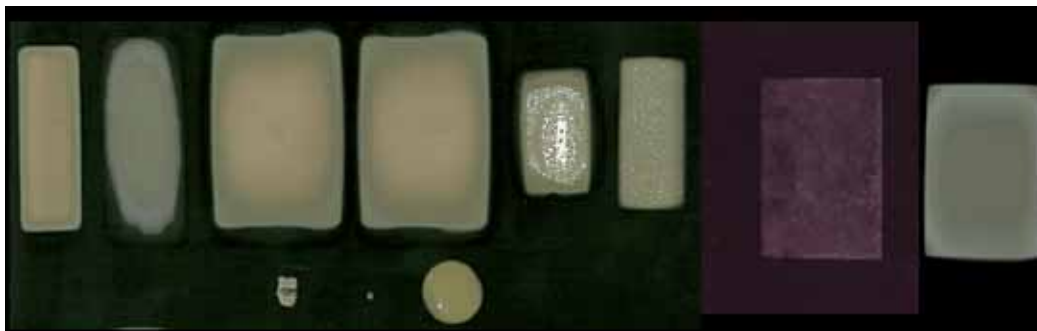
Fig 4. Spatial profile of measured systems (top left to right: Philips SatinLux Lumea, Dezak Rio IPL8000, HomeSkinovations Silk'n, HomeSkinovations Sensepil, Remington i-Light/LumaSmooth, CyDen iPulse Personal; Bottom left to right: Dezac Rio Scanning Laser Hair Remover, Dezac Rio Laser Hair Remover, Tria Beauty, Tria) showing the diode lasers have relatively small treatment areas and the histograms indicate poor energy distribution for some of the IPL devices.
