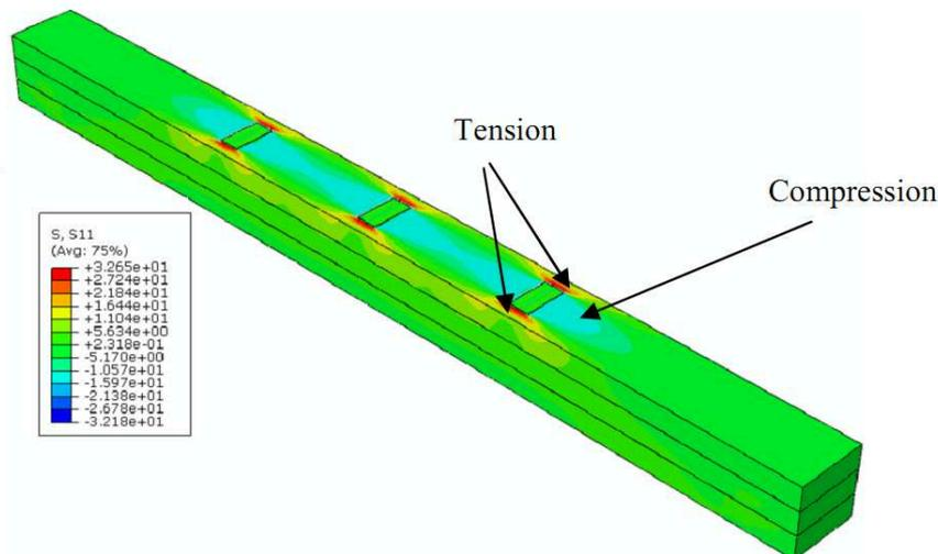
Figure 4: Bending stress (MPa) distributions around the CW block for beams reinforced by three CW 30 mm thick.
