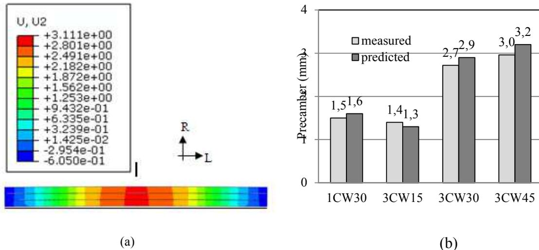
Figure 2: (a) Modelling of pre-camber (mm) for a beam reinforced by three 30mm thick CW blocks, (b) Comparison of the simulated and measured pre-camber deflections for beams reinforced.
