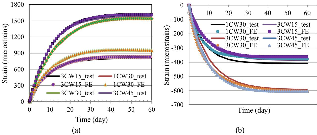
Figure 3: Comparisons of the predicted and measured tensile and compressive strains at the top and the bottom extreme fibre of the beams pre-stressed.
