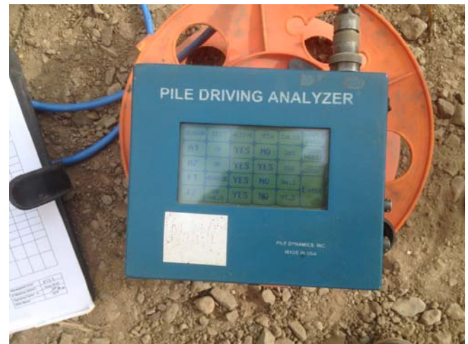
Figure 2. Pile Driving Analyser: an accelerometer and strain gauge pair for measuring transferred energy on a DCIS pile tube (top), data acquisition unit (bottom)
