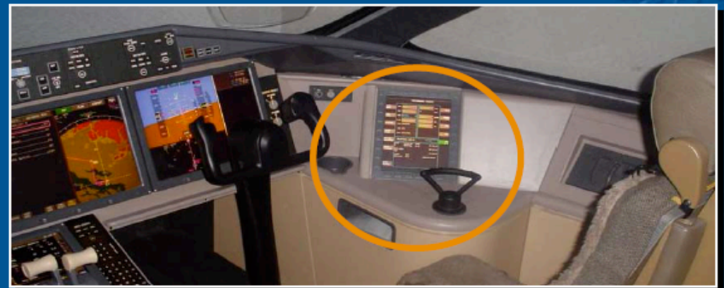
Figure 2.16. The Electronic Flight Bag on a Boeing 787 Flight Deck. Source: Carriker, 2006.
