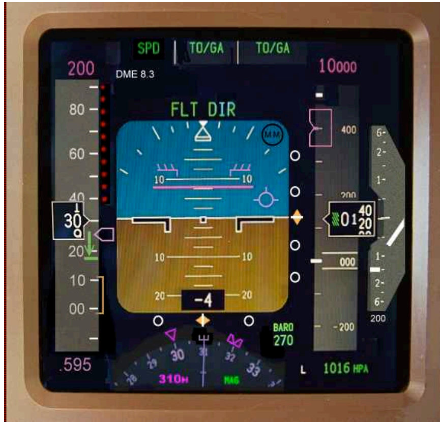
Figure 2.5. A Primary Flight Display
