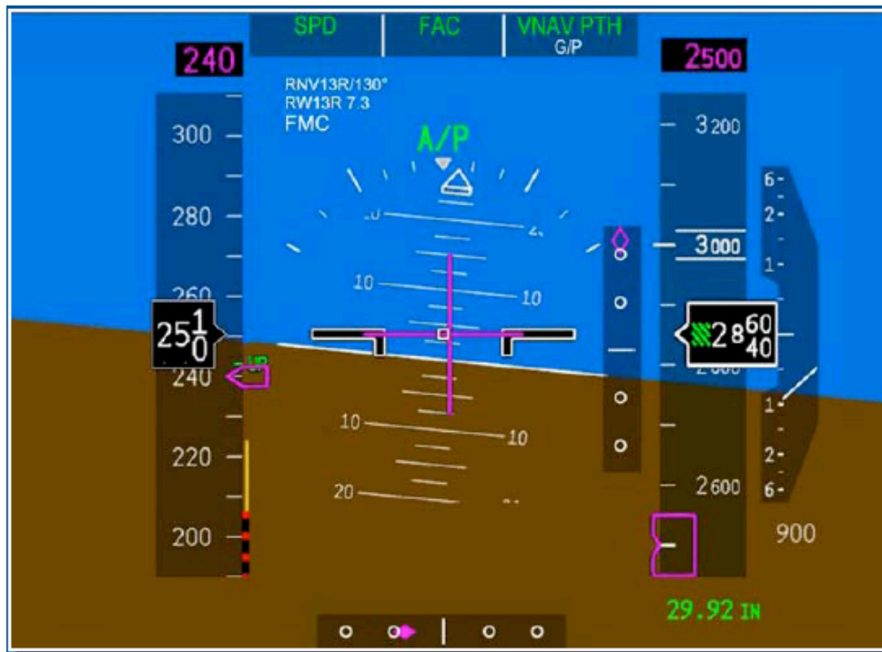
Figure 2.18. A potential PFD with integrated navigation performance data. Source: Carriker, 2006.
