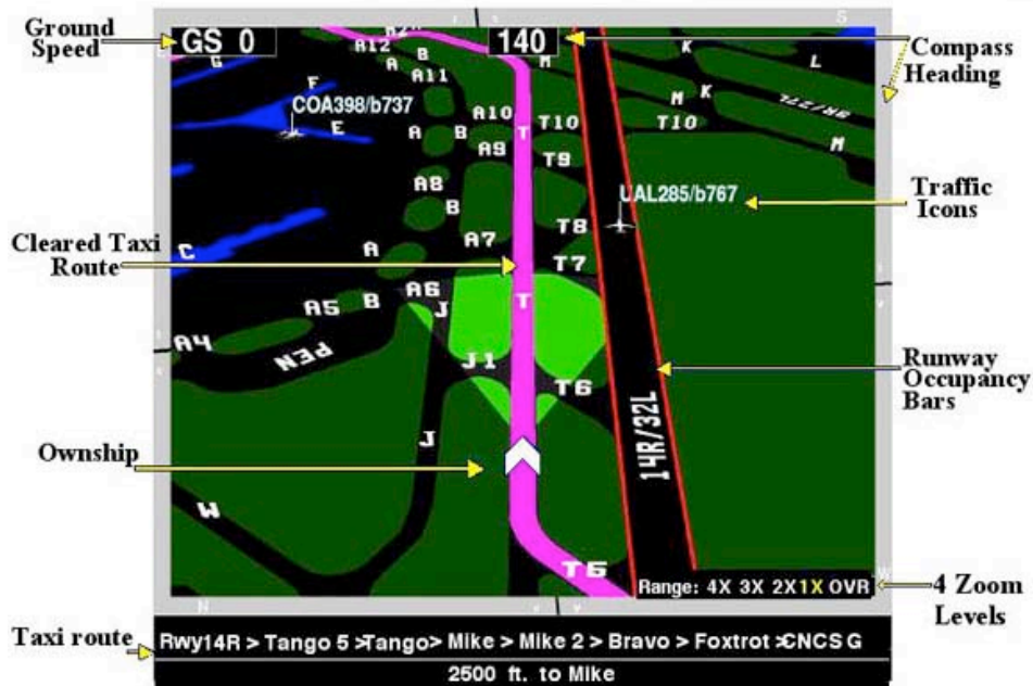
Figure 2.17. A Potential Surface Map Display Taxiway Navigation and Situation Awareness (T-NASA) Display. Source: Hooey, Foyle, & Andre, 2002.
