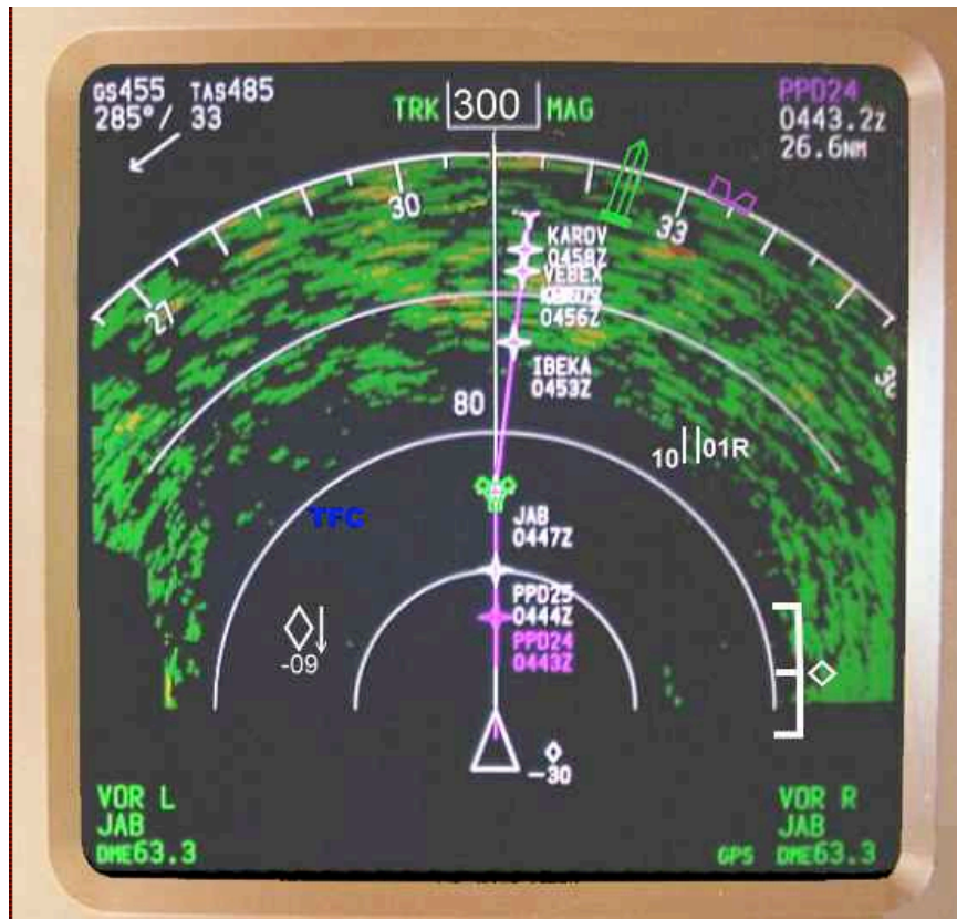
Figure 2.6. A Navigation Display
