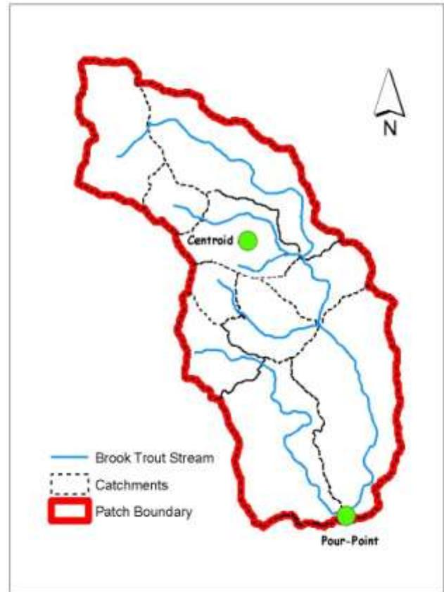
**Figure 1. Contiguous catchments containing brook trout were dissolved into “patches” of reproducing brook trout habitat. Paired air and water temperature thermographs were placed at pour point and at the stream section nearest to the centroid to directly measure water temperature responses to air temperatures.**
